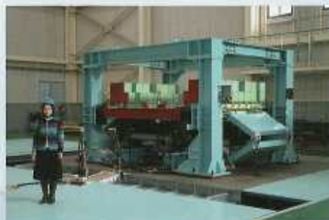
▲ Large-scale vibration test machine
