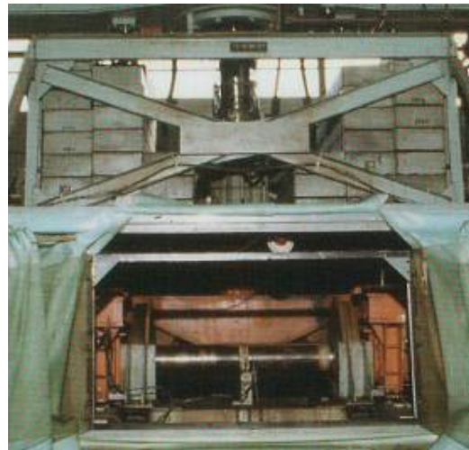
Wheelset fatigue testing machine
