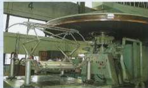
▲ Pantograph testing equipment
