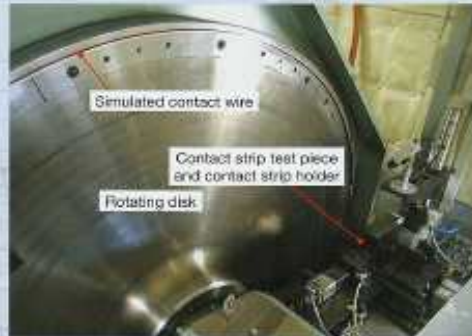
▲ Wear test machine for current-collecting materials for high-speed railways
